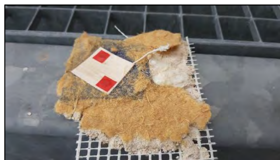
Figure 45 : Removed render layer of variant N 2.6 (dark render) with Balsa sensor and wood fibre residues: No fungal mycelium visible.
