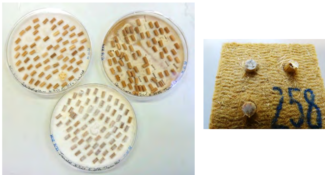
Figure 26 Preparation of infected wooden dowels (left: Schizophyllum commune , top right: Coniophora puteana , bottom: Trametes versicolour ) and specimen "inoculated" with dowels.
